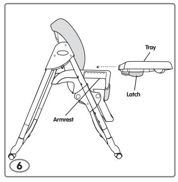
• While pulling the latches underneath the tray out, slide it onto the armrests. Release the latches to secure the tray in place.
